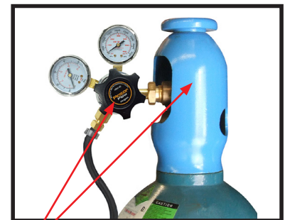
(14) Carefully open the valve of the gas cylinder, set the flow to 11-21 cfh.
